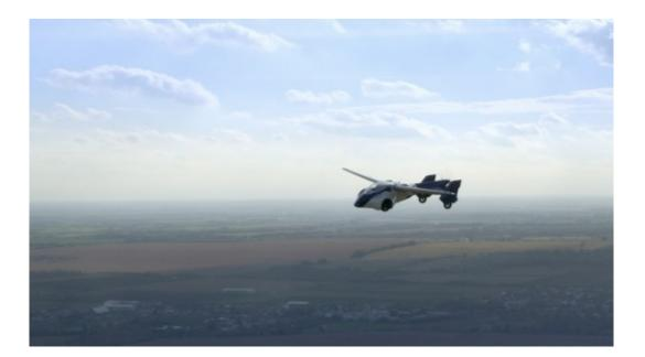
The new prototype was designed by Klein and the company's other co-founder Juraj Vaculik. It is built from predominantly the same materials as will be used for the final product and has all of the main features that will be present. These include avionics equipment, autopilot and an advanced parachute deployment system.
